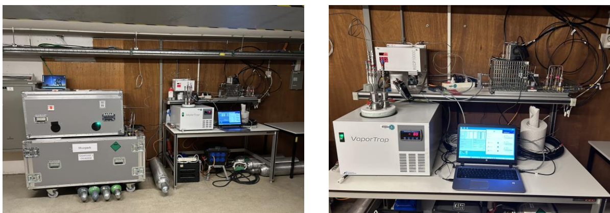
Fig. 5: O 2 and CO 2 instrument setup. Showing the instrument and cylinder flight case and the vapor trap, cooler and heights valve system.
