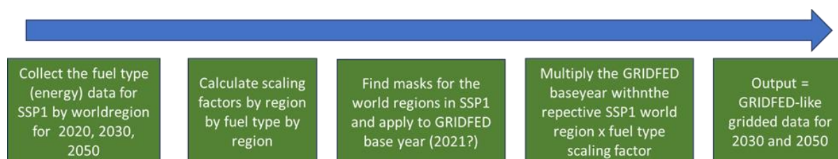
Figure 7.3: Workflow to derive APO grid maps for future years (2030 and 2050) based on gridded GridFED APO data for the present (2019-2021).
